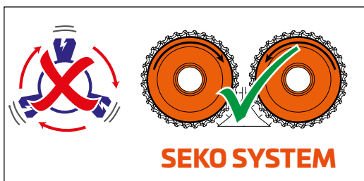
The low rpm grant a high output and a low wearing of the blades and all wearable elements
