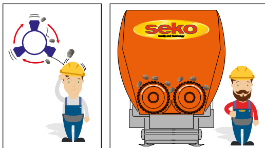
Seko system, at low rpm, avoids throwing products within the working area
