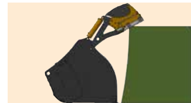
Loading the top of the clamp: patented deflector in low position
