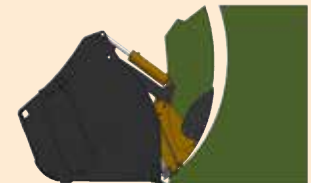
Loading the bottom of the clamp: patented deflector in high position
