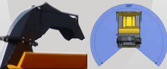
260° swivel chute to spread between 15 and 20m
