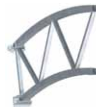
The truss arch enlarges the span width by optimizing material. The best technical choice for spans greater than 15 m.
