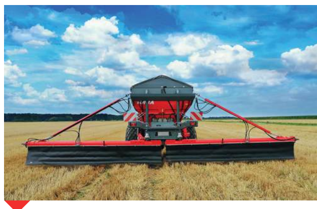
Beam for spreading lime powder
