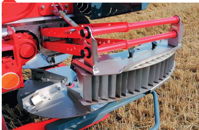
Mechanically or hydraulically foldable limiter for border spreading
