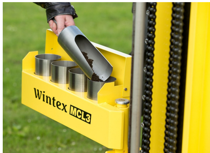
The soil is removed from the probe and filled into the soil bins with a sampling scoop and a scraper.
