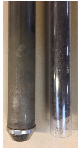
Extras: a custom-made probe with an integrated plastic liner makes it possible to extract and keep a whole core of soil.
