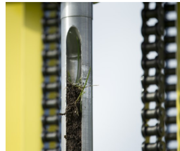
The probe goes into the ground by the means of a high-frequency hammer.
