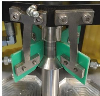
The scraper fits the inner diameter of the probe precisely, and the scraper blades ensure that the probe is emptied fully before going into the ground again.
