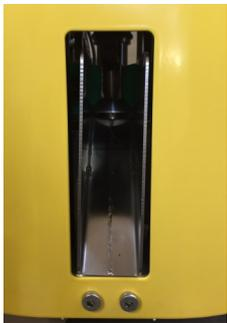
If the **WINTEX 3000** meets obstacles or is interrupted during the sampling proces and therefore takes an incomplete sample, the sample will be discarded through a funnel and will not be filled into the soil boxes.
