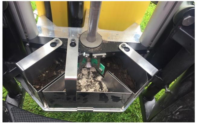
Soil from different layers is automatically filled into the soil boxes. Dividing the samples is conducted with close accuracy.
