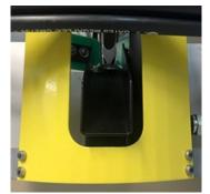
If the **WINTEX 2000** meets obstacles or is interupted during the sampling proces and therefore takes an incomplete sample, the sample will be discarded through a funnel and will not be filled into the soil boxes.
