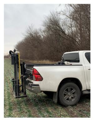
The **WINTEX 2000** can be mounted on a wide range of carrier vehicles, for example ATVs, UTVs, tractors, pick-ups, low tonnage vans and trailers.
