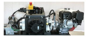
The custom-made oil tank is made of aluminum. It has a ribbed surface which means that the area of the oil tank is three times larger than a plain surface. Because of the aluminum and the ribbed surface the cooling capacity is 12 times higher than the cooling capacity of a traditional oil tank, ensuring optimal cooling of the hydraulic oil.
