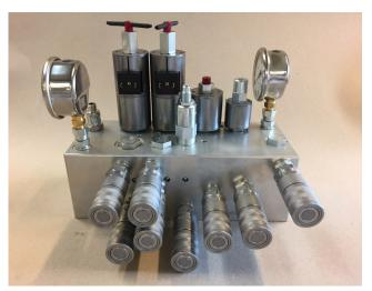
All functions are conducted by the custom-made distribution block. The hydraulic system has a simple construction which makes maintenance easy and uncomplicated.
