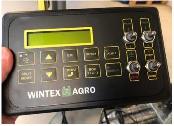
All actions can be carried out from the control system. Pre-settings like the depth, sticks and layers per sample as well as choosing the soil box can quickly and easily be entered into the the control system.
