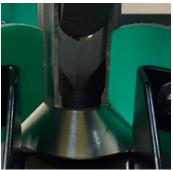
The scraper fits the inner diameter of the probe precisely, and the scraper blades ensure that the probe is emptied fully before going into the gound again.
