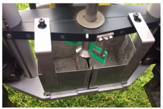
Soil from different layers is automatically filled into the soil boxes. Dividing the samples is conducted with close accuracy.
