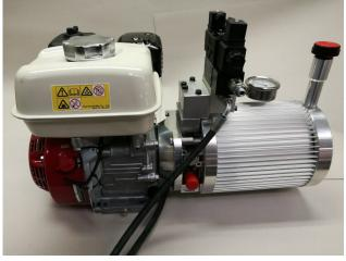
The custom-made oil tank is made of aluminum. It has a ribbed surface which means that the area of the oil tank is three times larger than a plain surface. Because of the aluminum and the ribbed surface the cooling capacity is 12 times higher than the cooling capacity of a traditional oil tank, ensuring optimal cooling of the hydraulic oil.
