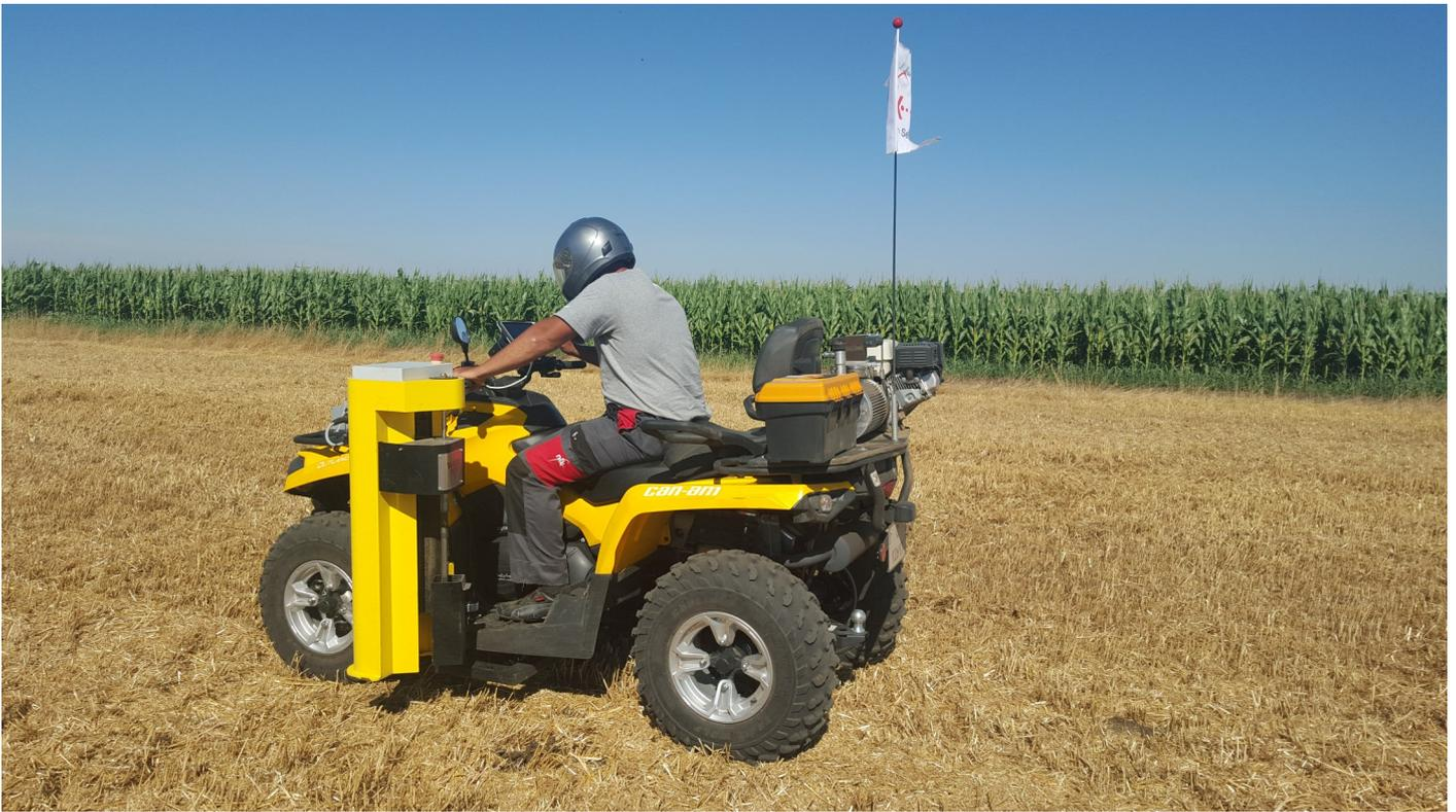
The **WINTEX 1000** is an efficient and strong automatic soil sampler for soil samples up to 25 cm. It is user-friendly, requires only minimum maintenance and is easy to use. All functions are comfortably carried out from the driver's seat.
