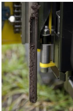
The probe is easily replaced, even in the field. Just loosen the lock nut, and mount the new probe.
