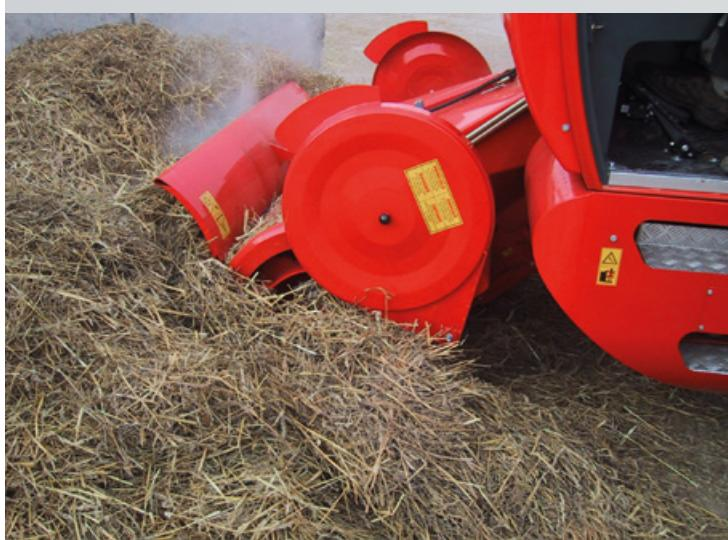
Wide tillaging arm channel for high loading capacity with continuous rubber belt (without any joint hinge) for longer life.
