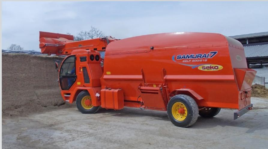
Tillaging roller diameter 400 mm, driven by 1 hydraulic motor power 100 kW, equipped with a large number of different geometry blades for maximum efficiency even in the collection of loose products on the ground such as flours, fodder and other supplements.
