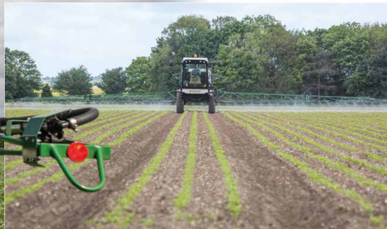
Dual or quad nozzle set-ups reduce boom pressure and drift
