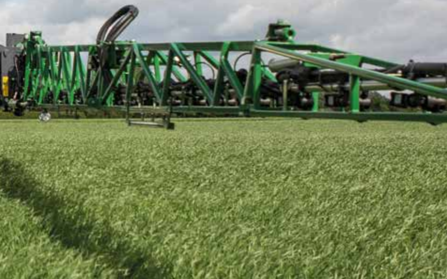
Dual or quad nozzle set-ups reduce boom pressure and drift
